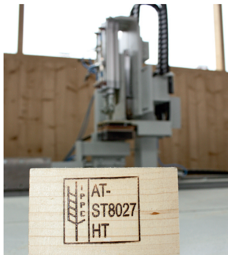
The IPPC logo can be branded onto the pallet blocks thanks to the branding iron (in the background)
