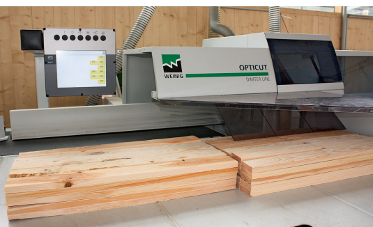
On the outfeed monitor, the operator can watch the dimensions related to the corresponding order
