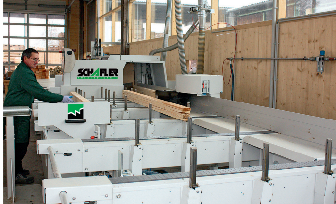
The operator puts the raw lengths (max. 6,3 m) onto the table from where they are automatically introduced by catch series
