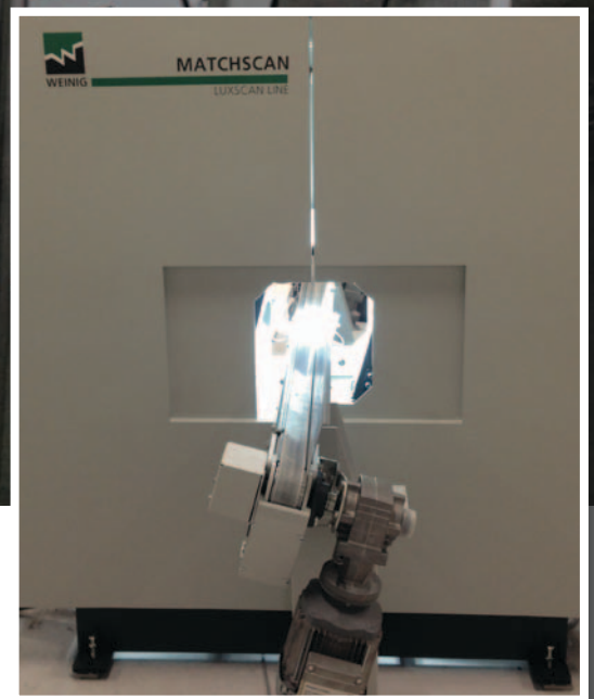
The colour-sorting scanner for Tiger Excellent Wood Sdn Bhd
